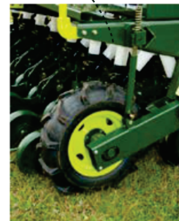
Wheel with pressure adjustment option using a spring and chamber.
