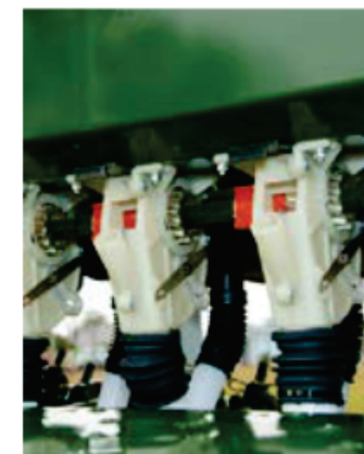
Seed distribution by means of a steel helical rotor.
