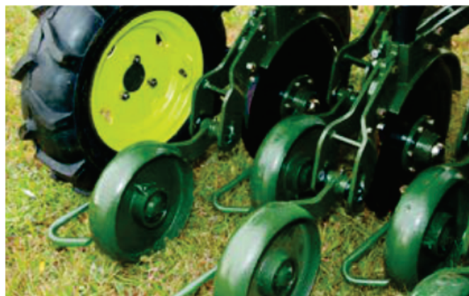
Consisting of offset 15x15" double discs and optional cast iron compression. Ring system, standard item.
